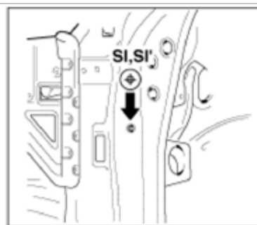
Front door checker mounting hole (ø1)
