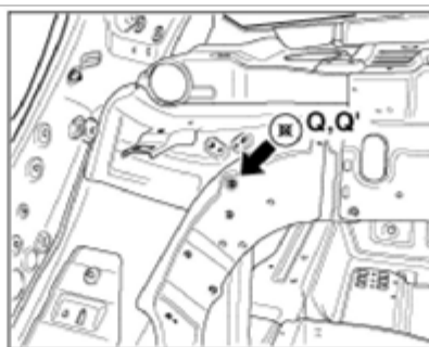
Quarter inner panel tooling hole (ø9)
