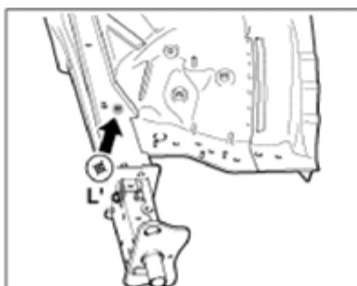
Front side member tooling hole (RH/LH-ø7/ø11)
