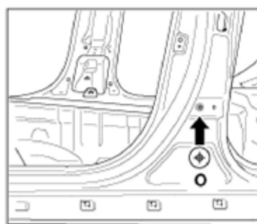
Rear door hinge lower mounting h hole (ø11)
