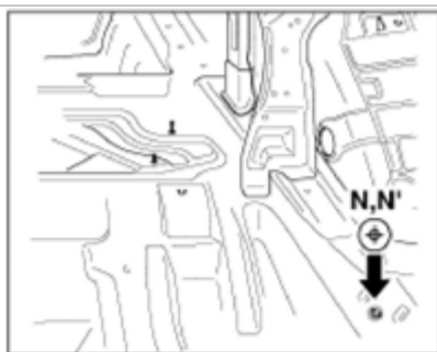
Floor panel tooling hole (ø12)
