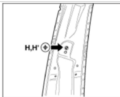
Seat belt height adjuster mounting hole (ø13)
