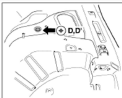
Shockabsorber housing panel tooling hole (ø20)
