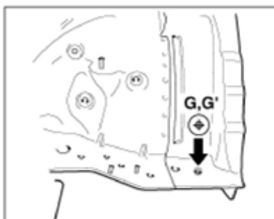
Fender apron panel tooling hole (ø7)
