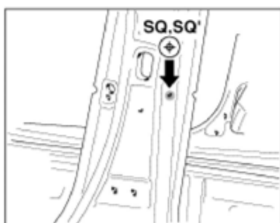
Rear door checker mounting hole (ø11)
