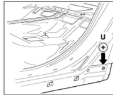
Side garnish mounting hole (12X1)
