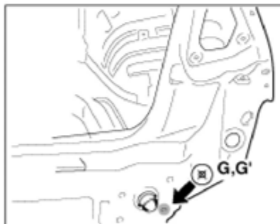
Back panel tooling hole (ø8)
