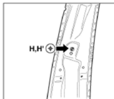
Seat belt height adjuster lower mounting hole (ø1)
