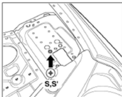
Package tray panel tooling hole (ø10)
