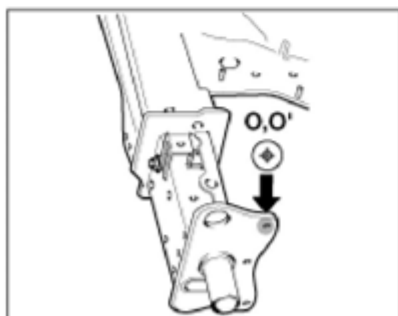
Crash member bracket tooling hole (ø9)
